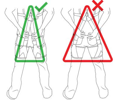
Adjust thigh sleeves so the bands pass over the middle of each buttock. Bands should not be rotated too far to the outside of the hips.
