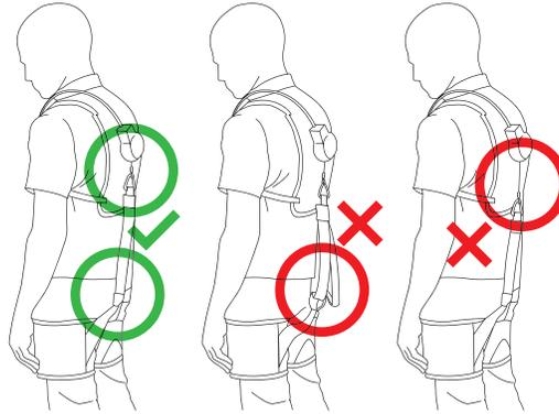
When standing upright with the suit 'off', the bands should not be slack or loose, and there should not be more than 2 inches of rope extending from the clutch.
