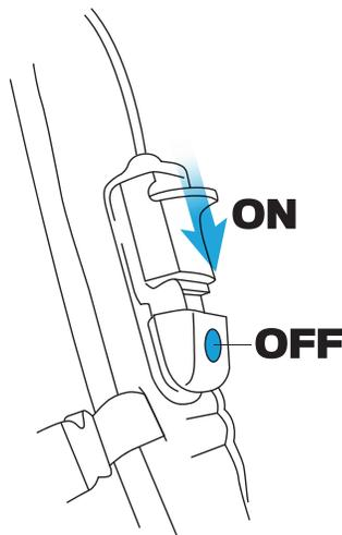
Engage the system by pulling down on the upper portion of the Switch until it clicks.
